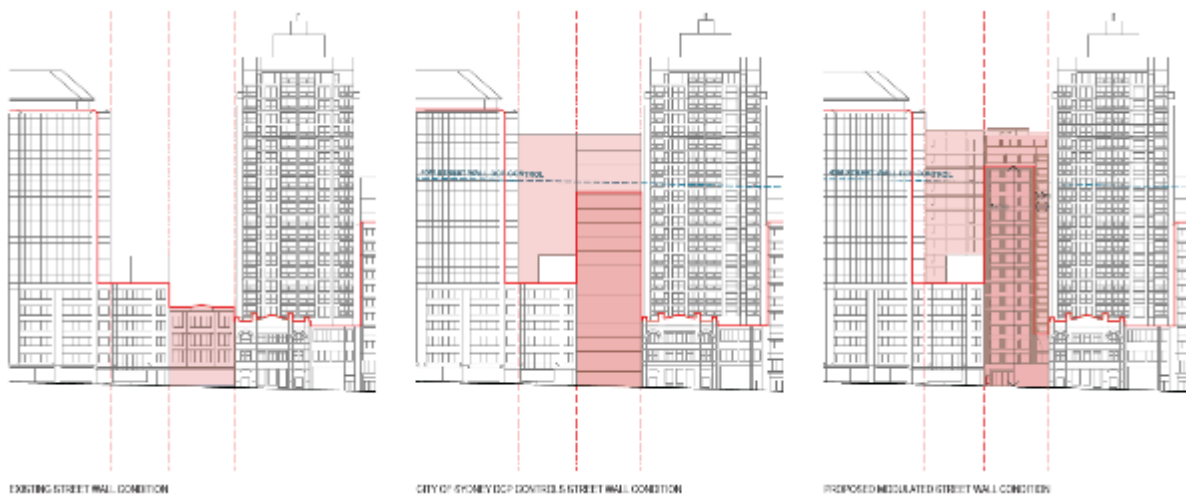
Figure 47: Street wall analysis of eastern side of Castlereagh Street, showing the existing site, the DCP compliant built form and the proposed development
