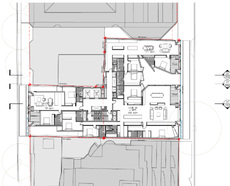
Figure 17: Originally lodged scheme - Typical 9-12 level floor plan
